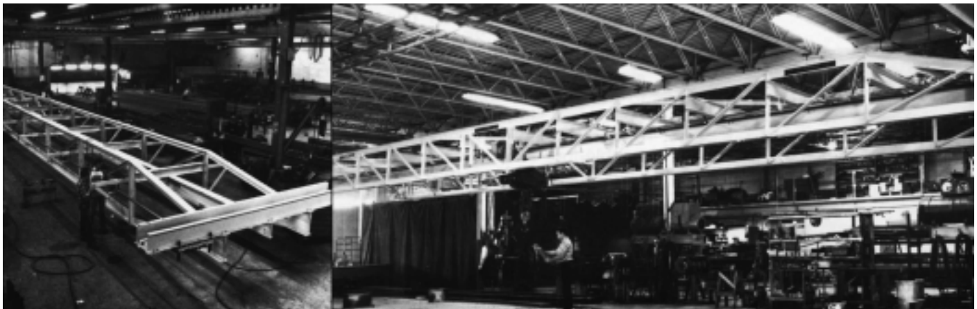
Above left: A single girder, double truss crane is manufactured in the shop. Above right: A view of a single girder, double truss crane in a manufacturing shop. Note the crane structure with the two trusses, the single bridge girder and the associated framing. This crane provides excellent floor coverage with a full-load rating while working in a shop with ceiling height restrictions.
