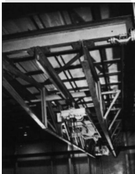
End view of crane. Tractor, tow bar and two twin hook hoist units visible on center bridge beam form a unit with 4 hooks spaced at 25'0" to pick up a long load.
